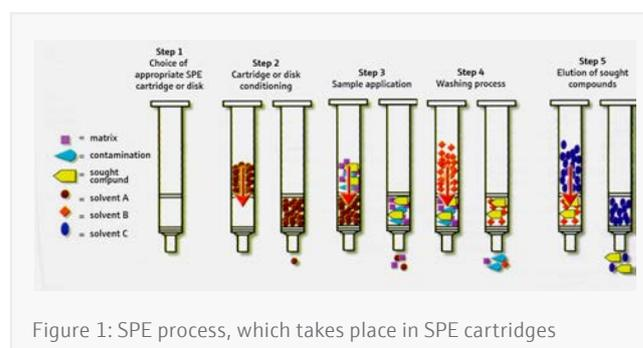
Figure 1: SPE process, which takes place in SPE cartridges
