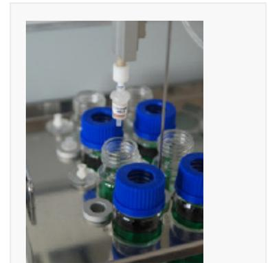
Figure 2: APU 28 SPE sample rack
