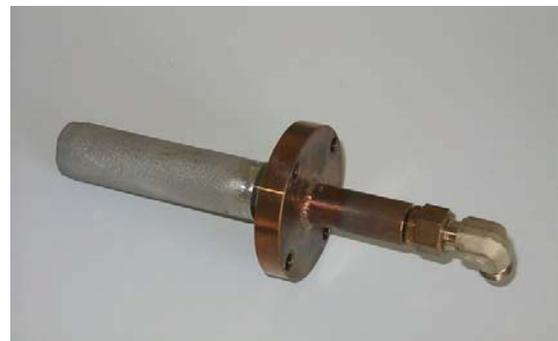
Fig. 3: Amalgamation of mercury on a gold trap
