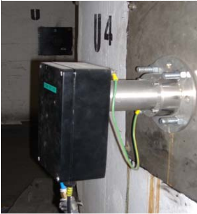
In situ version of light scatter used on FGD with reheat
