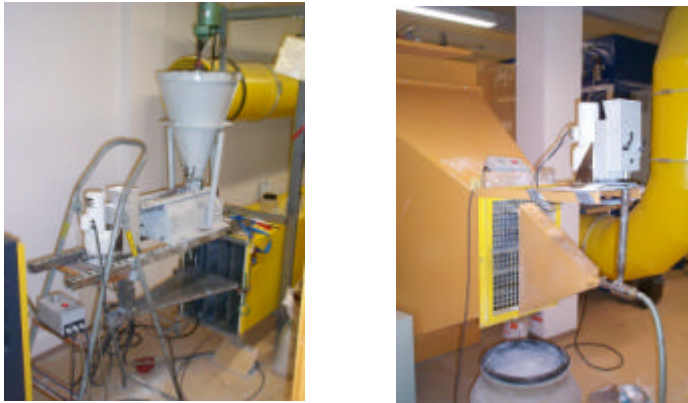
Figure 1 : Dosage system (dust feeder)
