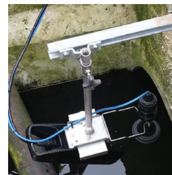
Other choices include ultrasonic flow meters, Time of Flight Flow meters, Insertion Flow Meters & non contact flow velocity meters (last two pictured)
