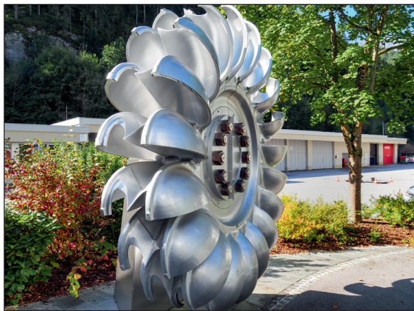
This Pelton turbine in front of the central control room in Mayrhofen is a typical piece of equipment in the hydroelectric facilities in Tyrol. However, Pelton turbines are not used in every single one of the power stations.
