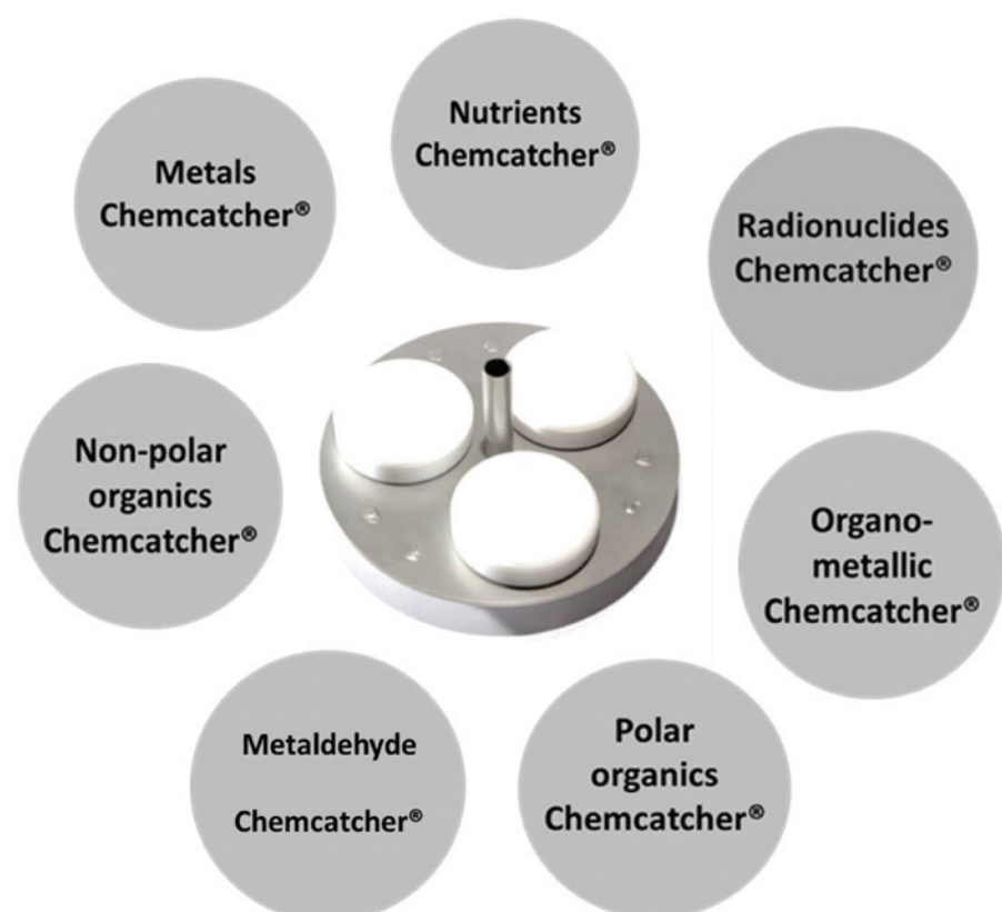
Fig. 3. Schematic of the different versions of Chemcatcher® for monitoring various types of environmental pollutants.
