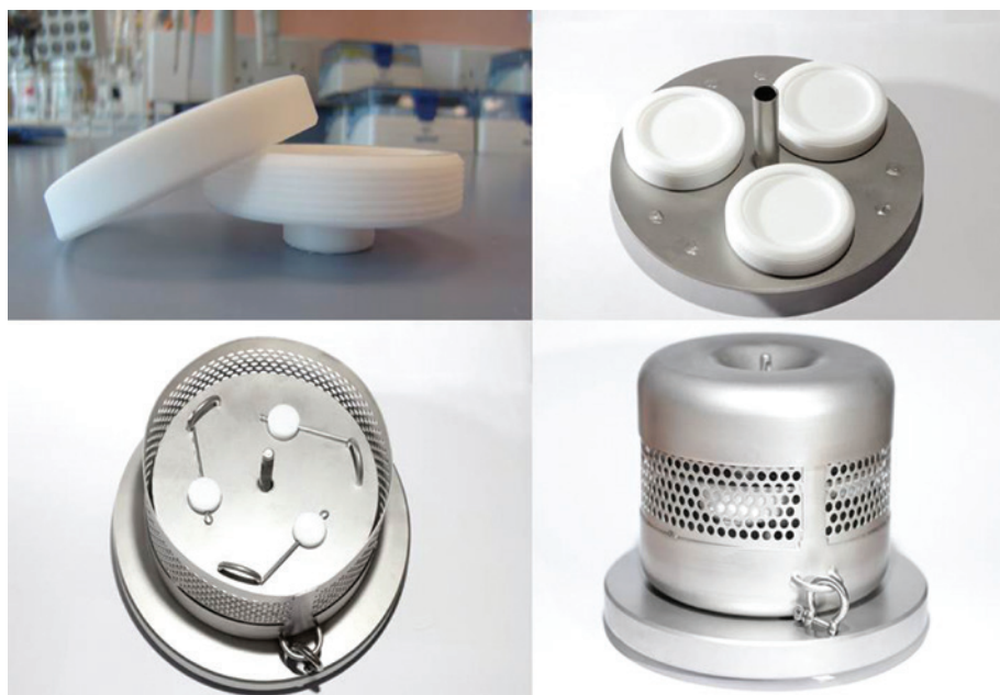
Fig. 2. Chemcatcher® passive sampler and a type of cage used for field deployments.
