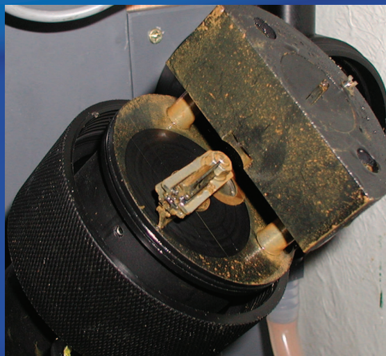
Fig.5: Suspended Solids Sensor showing the efficiency of mechanical wiping after six months operation.
