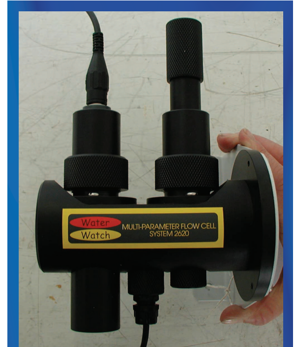
Fig.3: An integrated flow cell minimises the sample volume and maximises the ease of servicing.
