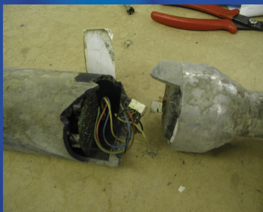
Fig.2: Terminal damage to a small 'sonde' after unexpected storm conditions.
