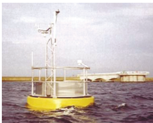
Photograph of a CEH buoy system on a water supply reservoir.
