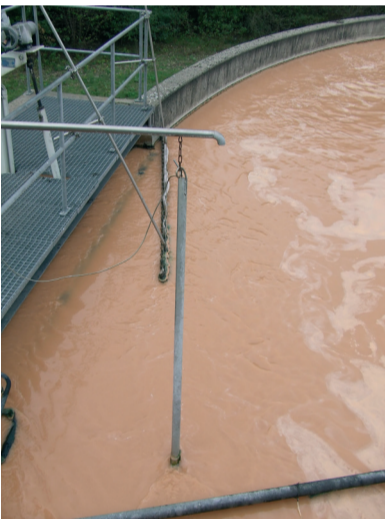
Fig. 2: LDO oxygen sensor in use
