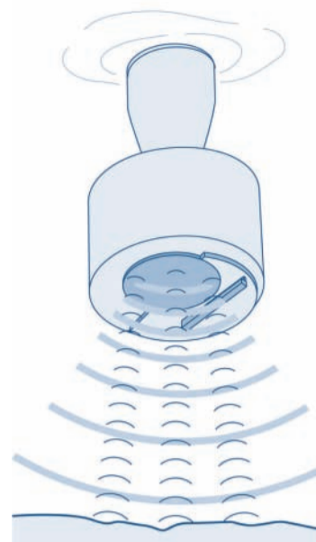
Fig. 6: The ultrasonic method and the mechanical wiper cleaning ensure reliable and stable measured values.
