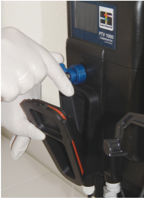
Pic. 3 : Air bubble trap with easy access from instrument front side
