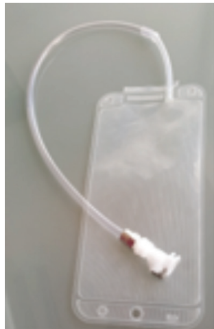
Pic. 4: TCalplus™ calibration bag with quick inlet coupling
