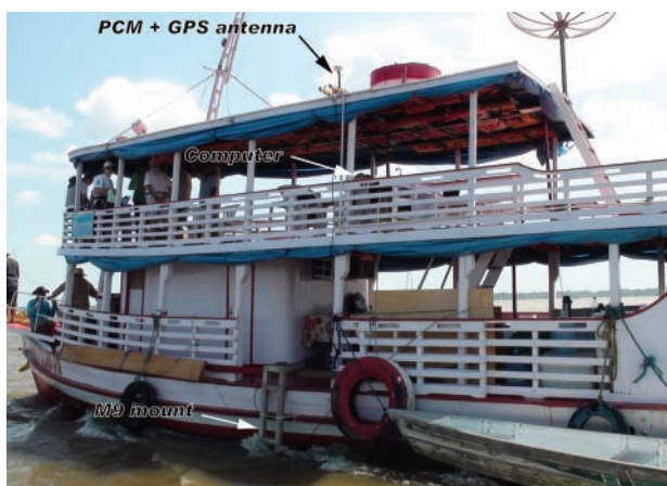
Figure 2: Boat used during the 2009 Amazon campaign. The Power and Communications Module (PCM) was secured to the roof of the vessel, along with the GPS antenna. The M9 system is in the water, about 1 m below the water line and attached to the boat with a custom-made mount. The computer on second deck received the processed data from the PCM via a Bluetooth radio link.
