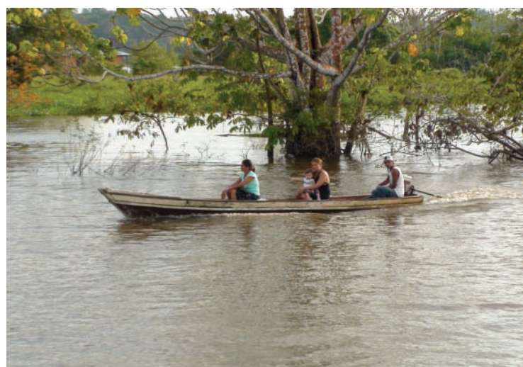
Figure 4: With practically no roads around, boats and other floating platforms are often the only means of transportation in this part of the world. A favorite of the local population, a minuscule outboard motor built from a gas-powered water pump—locally known as a "rabeta"—propels this family along the banks of the flooded Solimões river.
