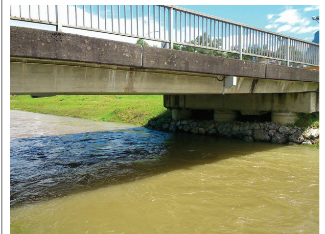
A monitoring station with an RQ at a canal with high water. No part of the station is submerged or in contact with the water, thus avoiding damage and providing maintenance-free operation.
