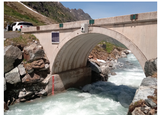
Measurement site with an RQ-30 at an Alpine river in Austria. It's primarily used to monitor snow melt in spring and early summer as one component of a flood warning and water management network. Monitoring stations high upstream extend the response time during potential flood conditions.
