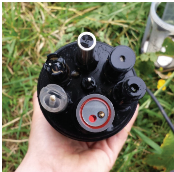
Eureka Manta2 – can now incorporate fluorimeters tuned for Tryptophan
