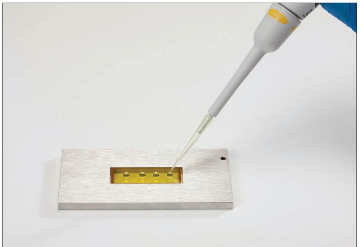
Figure 1: Sample deposition for the HATR method, constraining the sample to the most brightly illuminated portion of the crystal
