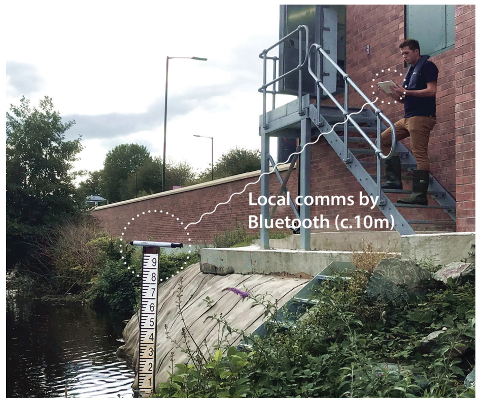
Local wireless communication with OTT ecoLog 1000 water level monitor improves the ease and safety of data management
