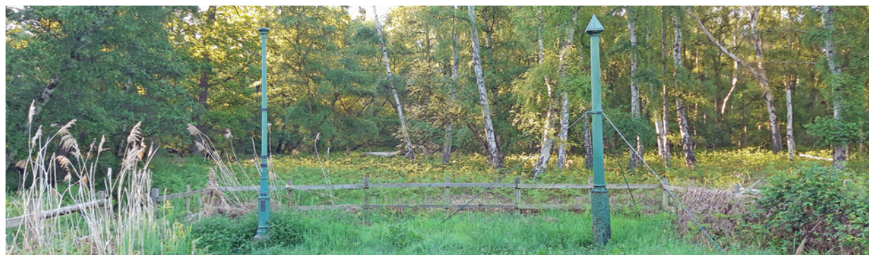
The Holme Posts were level with the ground in 1851, but are now 4m above ground due to peat shrinkage since the draining of Whittlesea Mere.
