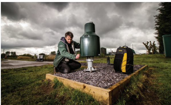
The OTT Pluvio 2 rain gauge is very accurate and reliable. Image courtesy of Barrie Scholes, Environment Agency.
