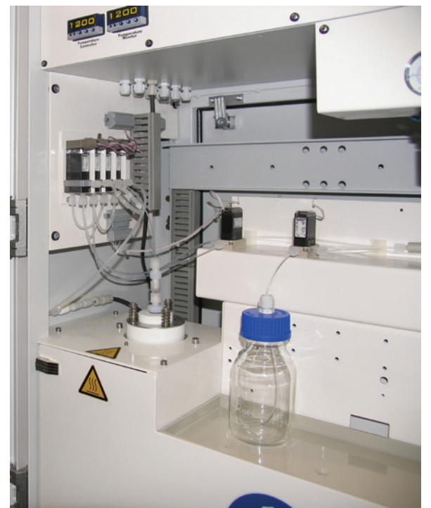
QuickTOCcondensate with inject loop and inlet for wet standards or grab sample
