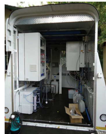
Figure 3: The mobile lab is equipped with state-of-the-art analysers and measurement methods and is able to automatically monitor 23 parameters in total.
