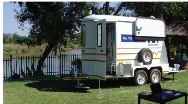
Figure 2: The online analysis and data transfer system has been practically implemented in form of a mobile laboratory that will be set-up at different measurement points along the Olifants River.
