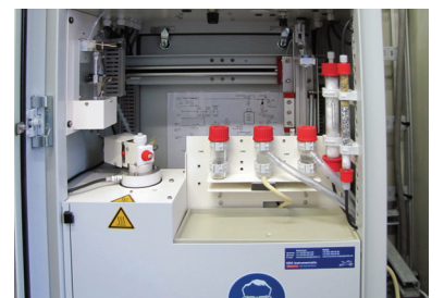
The QuickTOC uses a robot and only a few wetted parts
