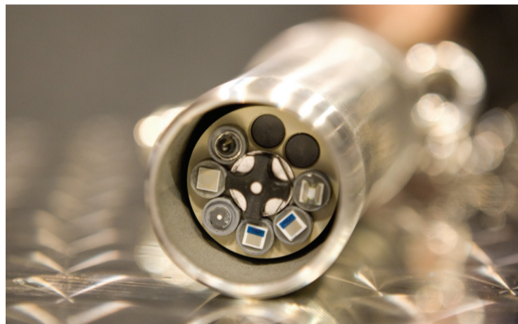
Up to 12 sensors inside a tiny sonde head
