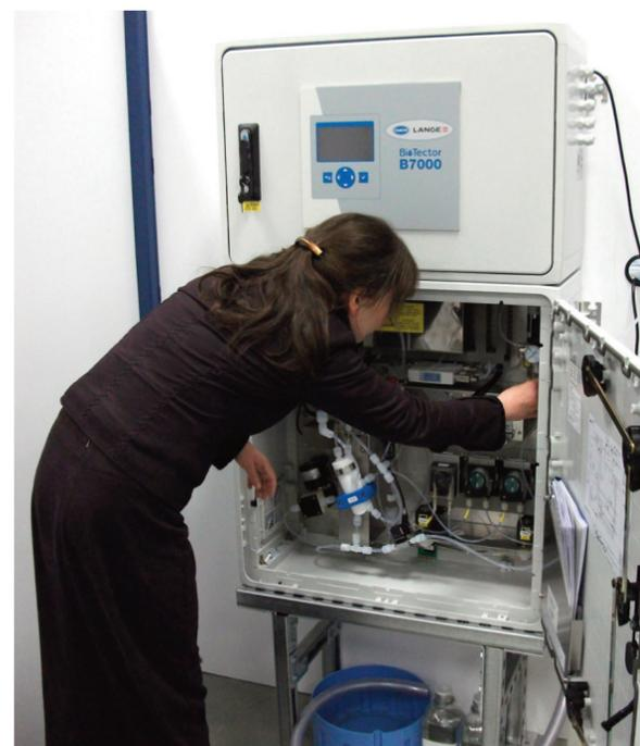
process personnel who can now see the effect that their activities are having on the effluent loads being discharged to the site treatment plant. Greencore has also linked the on-line results provided by the BioTector to an alarm system so that production personnel know when the TOC levels have increased - thus enabling them to react much quicker and thereby identify and address any issues as they arise."
