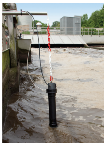
ISEmax used in the activated sludge basin of a municipal waste water treatment plant.
