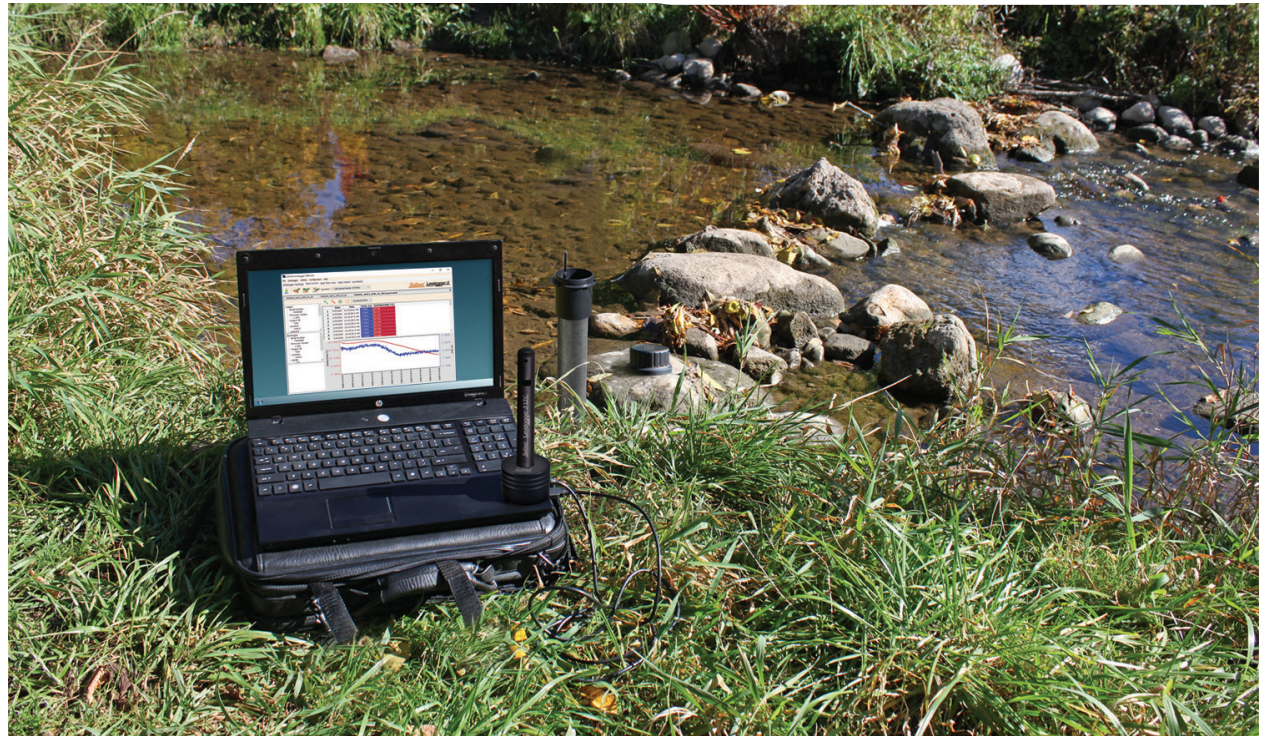
This is Levelogger 5 LTC (Water Level, Water Temperature, Water Conductivity) datalogger installed in a stream.
