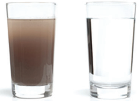
Cloudy and Discoloured Tap Water Caused by Turbidity
