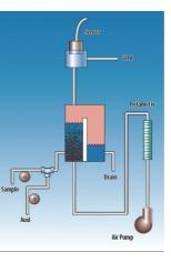
acid. In acid solutions chemical reactions lead to the production of H<sub>2</sub>S. The sample then flows to an air-stripping chamber. Measurement of gas phase H<sub>2</sub>S is carried out and the monitor displays an equivalent sulphide concentration in mg/l
