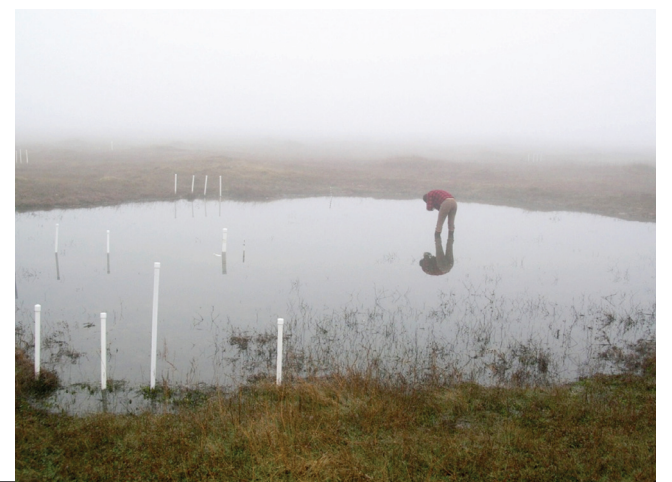
Vernal pool wetland near Sacramento, CA in wet season, with slotted PVC pipes containing water level dataloggers. (Courtesy of The Institute for Ecohydrology Research)
