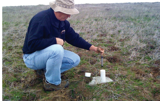
Installation of a Levellogger Junior at Beale Air Force Base as part of a wetland monitoring project for the U.S. Department of Defense. (Courtesy of The Institute for Ecohydrology Research)
