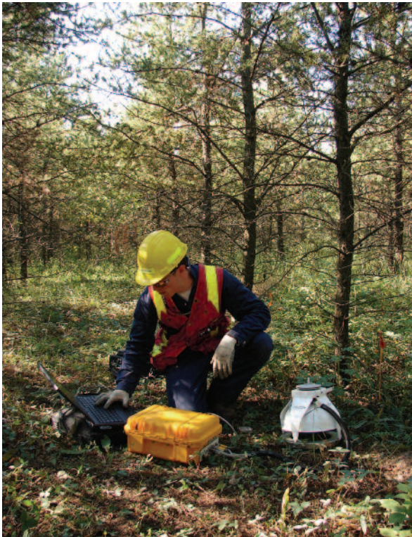
LI-COR's LI-8100A Automated Soil CO 2 Flux System deployed at a land reclamation site in the Athabasca Oil Sands Region of northern Alberta, Canada.
