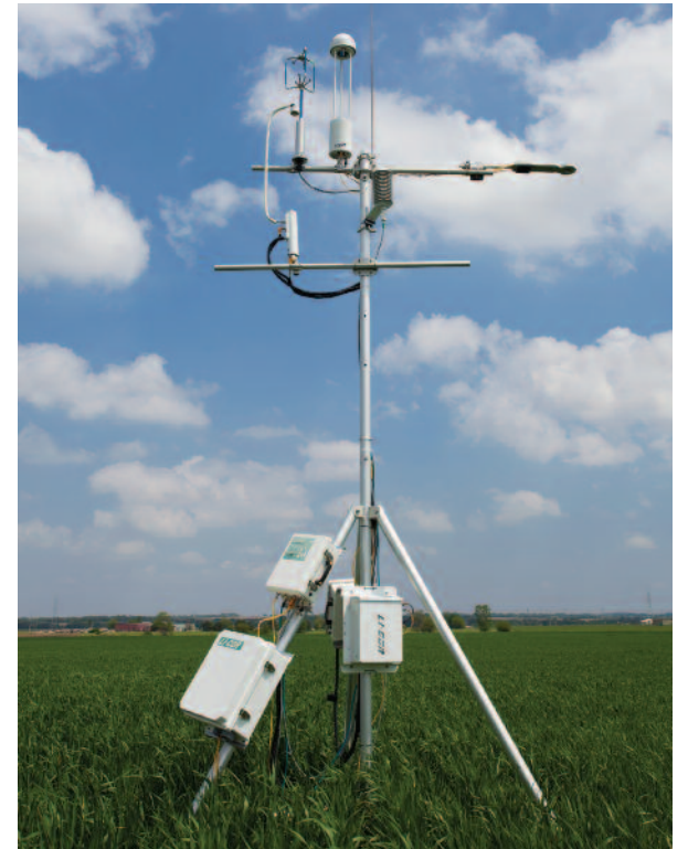
LI-COR's Eddy Covariance System equipped to measure CO 2 , H 2 O, and CH 4 fluxes.
