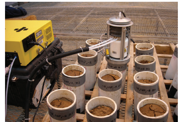
The DX4030 mobile-FTIR is seen (left) connected to a small soil flux chamber used to measure GHG emissions from PVC columns filled with soils amended with select rates of N fertilizer, sorghum residue, and a nitrification inhibitor in a greenhouse experiment.
