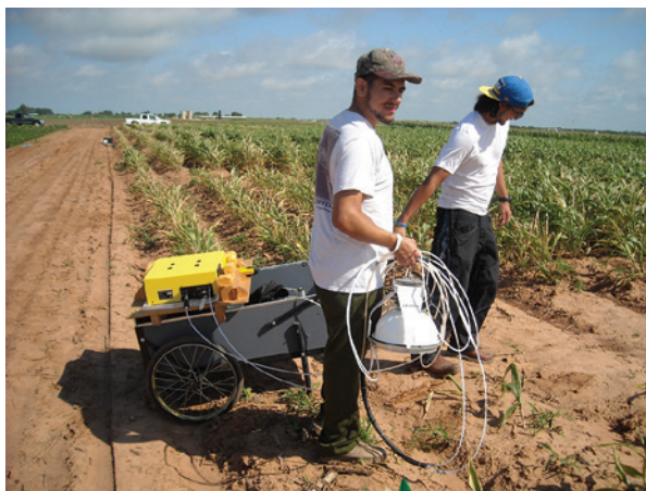
Student technicians Tony Guajardo and Chris Dermody wheel the DX4030 mobile-FTIR into position to begin measuring GHG emissions from the bioenergy sorghum fields.
