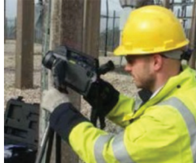
With the GF306, you can look at the switch gear equipment from a safe distance.
