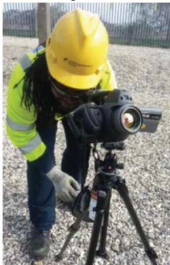
Thermal imaging cameras from FLIR allow SSEPD to detect possible leaks quickly and with high certainty.
