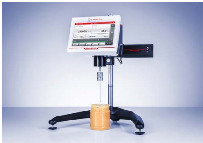
Figure 8: Rotational viscometer ViscoQC 300 with motorised drive and T-bar spindle for measuring non-flowing substances.
