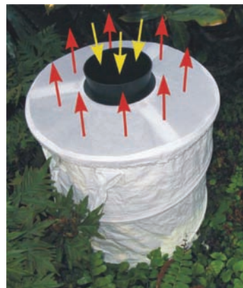
The yellow arrows show the direction of the drawn-in air, the red arrows the air loaded with the attractants which are emitted through the permeable fabric.
