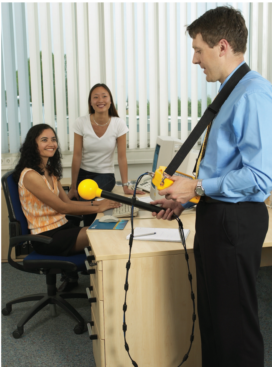
Fig. 1: Workplace overview measurement. The probe can be linked to the basic instrument by cable and held in the hand to make sample measurements throughout a room.
