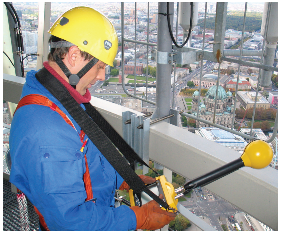
Fig. 4: Measurement of field exposure level for workers on a transmitting tower directly adjacent to digital radio broadcasting antennas (DAB).
