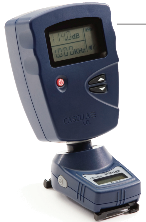
The CEL-350 dBadge being calibrated
