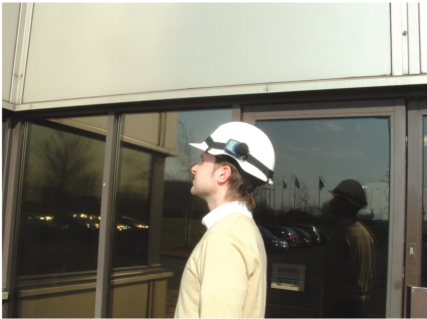
The CEL-350 dBadge mounted onto a hard hat
