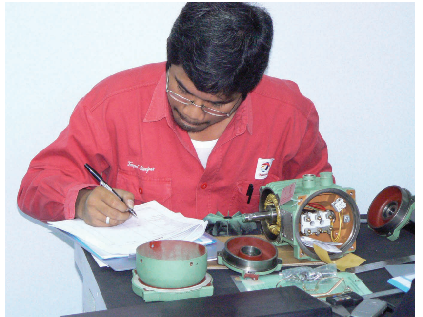
Examining a flameproof motor (courtesy AEMT)
