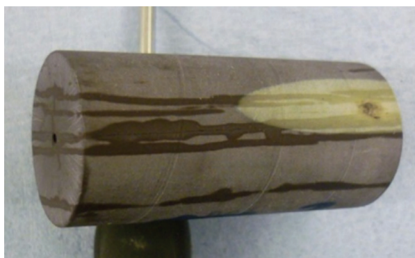
Figure 3: Hydraulic fractures produced in a laboratory specimen of slate. Fractures parallel to the length of the cylindrical sample (25 mm diameter) are oozing oil. The fractures were produced by injecting pressurised hydraulic oil into the specimen until it split apart on several fracture planes.
