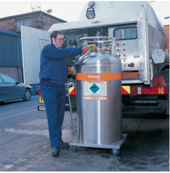
Liquid nitrogen is widely used and tanks are normally filled on site
