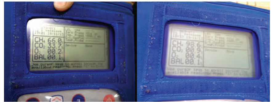
Geotech biogas analyser showing CH_4 upgraded from 66% to 98%
