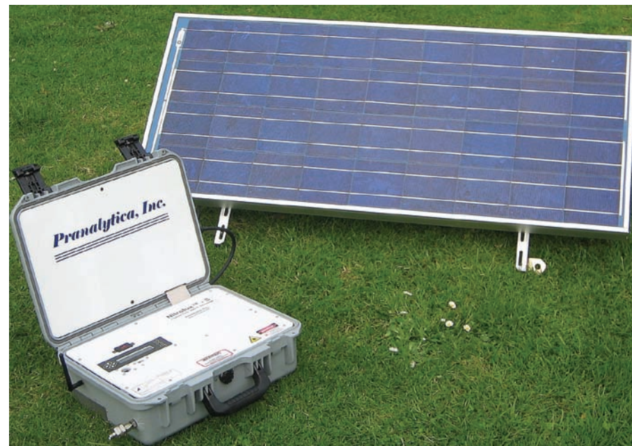
Figure 6. Nitrolux-S powered by an 80-W solar panel
