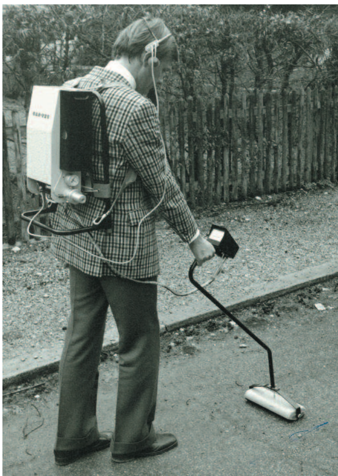
Gas detection has come a long way since the days of historic products like Gas Tec; a portable unit designed to detect underground gas leaks
