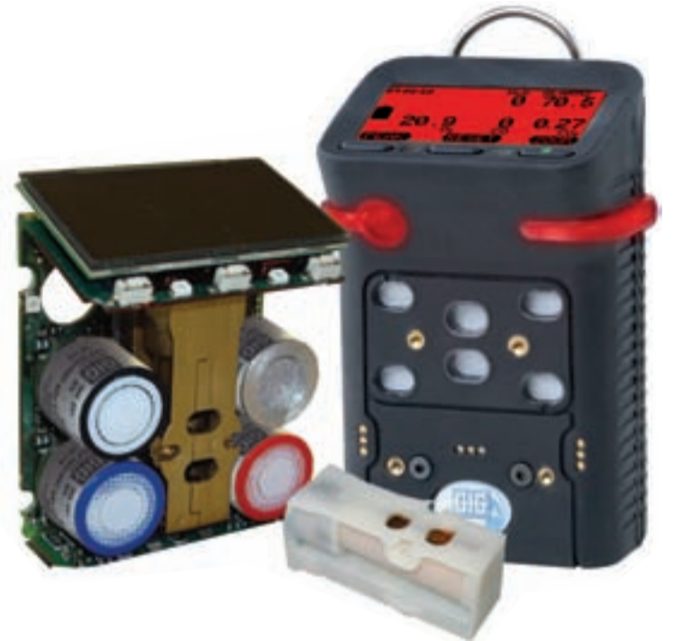
Multi-sensor instruments are able to use wide range of sensors and detection technologies including O 2 , standard pellistor LEL, NDIR combustible gas and CO 2 , PID and over 20 different substance-specific electrochemical sensors for toxic gas measurement
