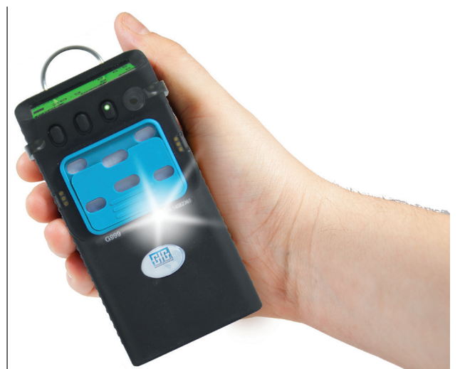
The G999 is a compact, one to six gas atmospheric monitor with optional wireless communication used to transmit real-time monitoring results to a remote collection point. The instrument is certified as an intrinsically safe “Ex i” device for use in Zone 1, gas group IIC, temperature class T4 hazardous locations.
