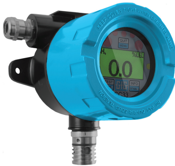
The CC-33 is a fixed system gas transmitter equipped with a catalytic LEL sensor. The transmitter is certified as a flameproof "Ex d" device for use in Zone 1, gas group IIC hazardous locations.
