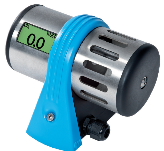
The IR-29 is a fixed system gas transmitter equipped with an infrared sensor used to measure LEL gas. The IR-29 is certified as an intrinsically safe "Ex i" device for use in Zone 0, gas group IIC, temperature class T4 hazardous locations. The sensor head of the low power transmitter can be removed and replaced while the transmitter is located in the hazardous location. The intrinsically safe design does not depend on an explosion proof housing, which reduces noise and improves performance of the IR sensor.
