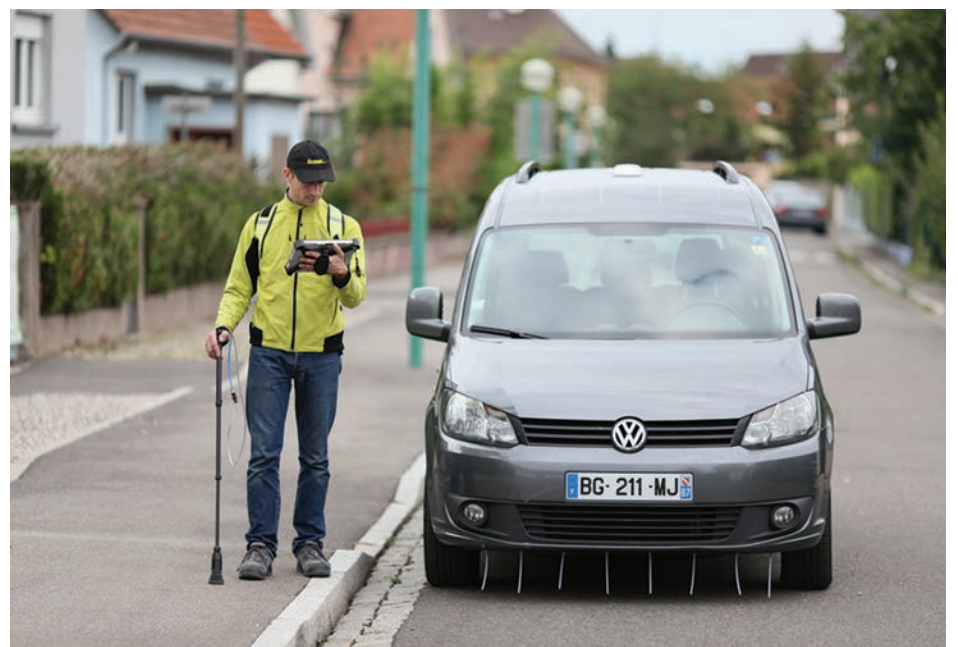
INSPECTRA® with operator and survey vehicle
