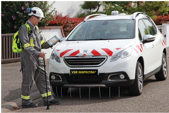
Network survey vehicle with on-board INSPECTRA system, GPS receiver and sampling system fitted under front bumper.
