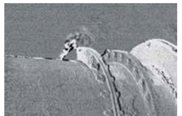
Natural gases like methane and ethane are clearly detectable with a mid-wave camera, like the FLIR GF320
