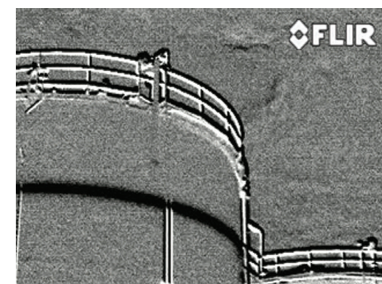
This thermal image taken with the FLIR GF320 optical gas imaging camera shows a leak in a tank containing piperylene, a flammable hydrocarbon which is produced as a byproduct of ethylene production from crude oil. The thermal image shows a leak as well as the liquid level inside the container.
