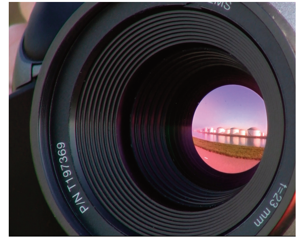
Optical gas imaging cameras can detect small leaks from several meters and big leaks from distances of hundreds of meters.
