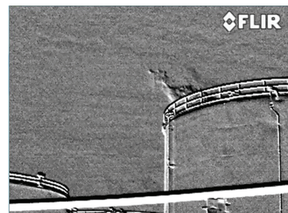
This thermal image taken with the FLIR GF320 optical gas imaging camera shows a leak in a tank containing a mixture of nafta and benzene.
