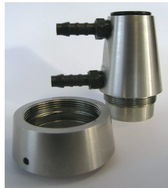
Figure 3: The two-part process cuvette in the Dräger Polytron IR
