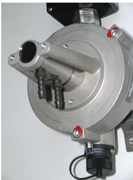
Figure 1: Dräger Polytron IR transmitter with newly designed process cuvette to shorten the t90 time
