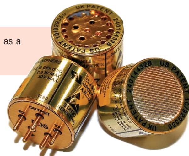
Figure 2: Miniaturised NDIR sensors directly measure CO 2 by means of absorbance of infrared light
